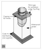
Code 4 lead flashing to be fitted at roof level as per Building Regulations. We recommend that you scorch a 5-10mm deep channel into the outer surface of the casings and fold in the top edge of the flashing.
