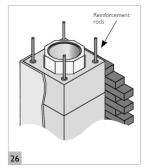
High tensile steel reinforcement rods will be required for all chimneys with a height that exceeds 1.4m above the roof line, 1.1m if the wind speed exceeds 44ms.
